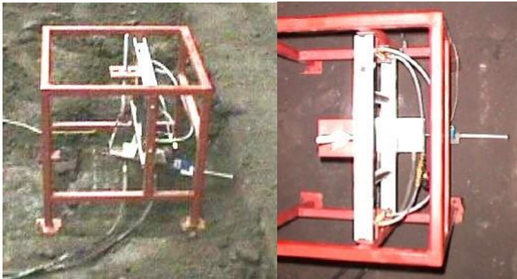
Figure 2. Apparatus supporting the cone penetrometer
